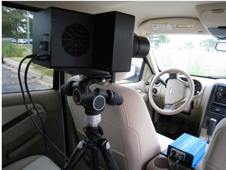
Figure 7. CCD Photometer from Driver's Perspective.
