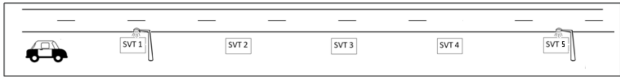
Figure 8. Luminance Measurement Layout.
