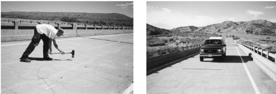
Figure 40 Methods of forced excitation of the Alamosa Canyon Bridge; (left) modal hammer and (right) flatbed truck driving over a wood stud place in the center of the span (after J. P. Lynch et al. [60])
