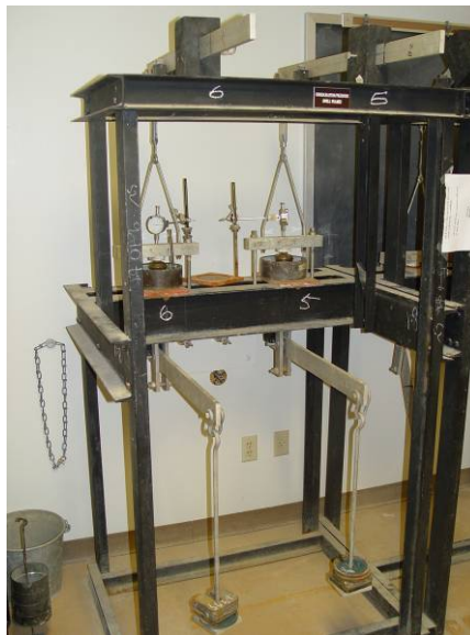
Figure 3.5 Constant volume swell pressure test setup.
