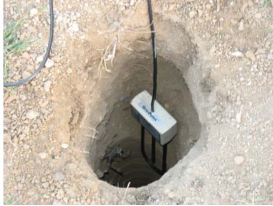
Figure 5.33 Field schematic of Gro-Point moisture probe installation.
