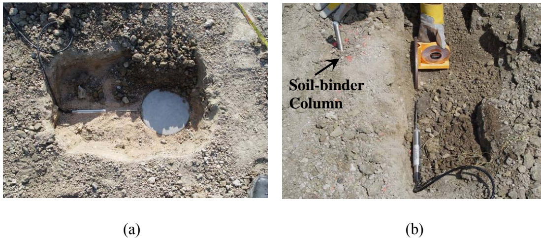
Figure 5.32 Schematic of pressure cell installation (a) Horizontal orientation and (b) Vertical orientation.
