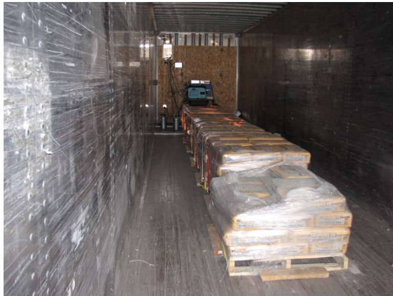
Figure 9. Photograph of Inside Testing Trailer with TTI's PEMS Units installed in the Front of the Trailer and Concrete Pallets Used to Simulate a Typical Load (The last pallet was removable to simulate a lighter trailer).
