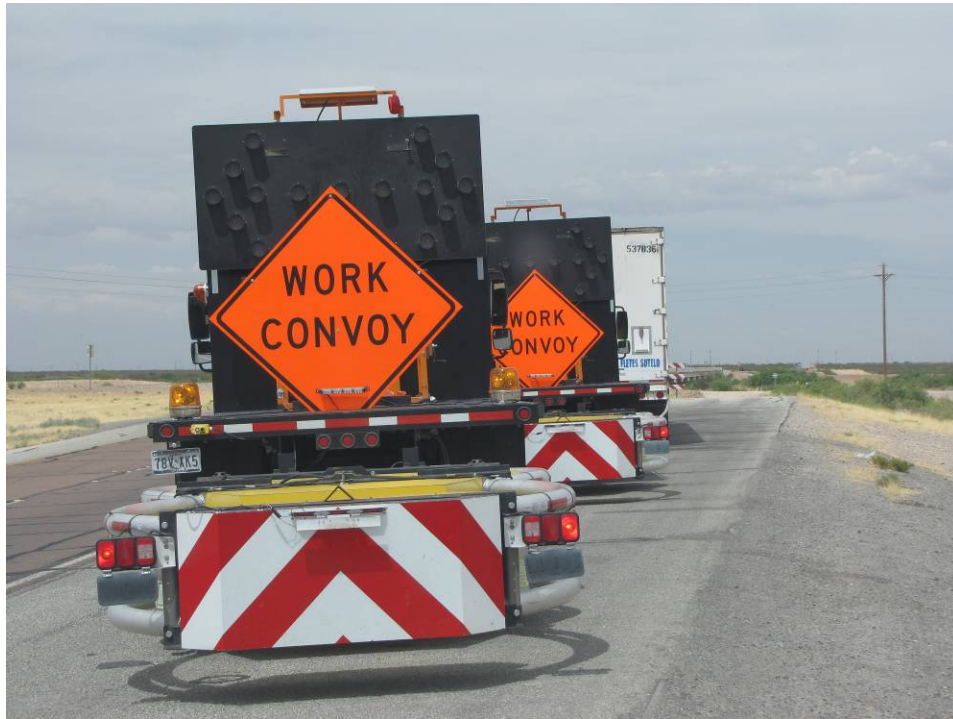
Figure 4. Photograph of Two Truck-Mounted Attenuators following a Drayage Truck during Testing to Warn Drivers of Atypical Conditions.
