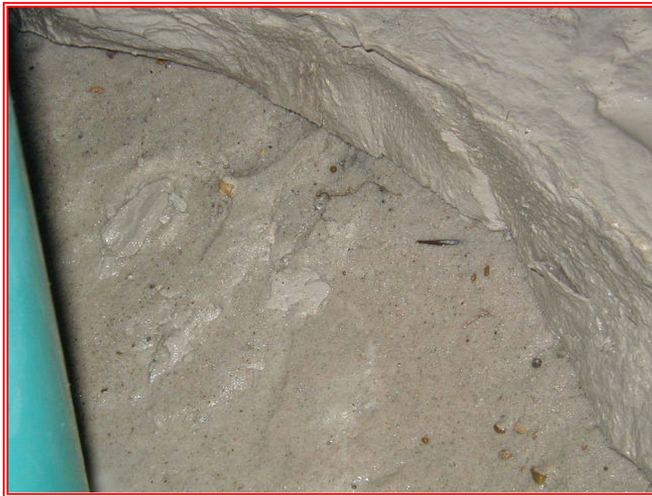
FIG 20 Steep Slope of the Scour Hole in Test 6
