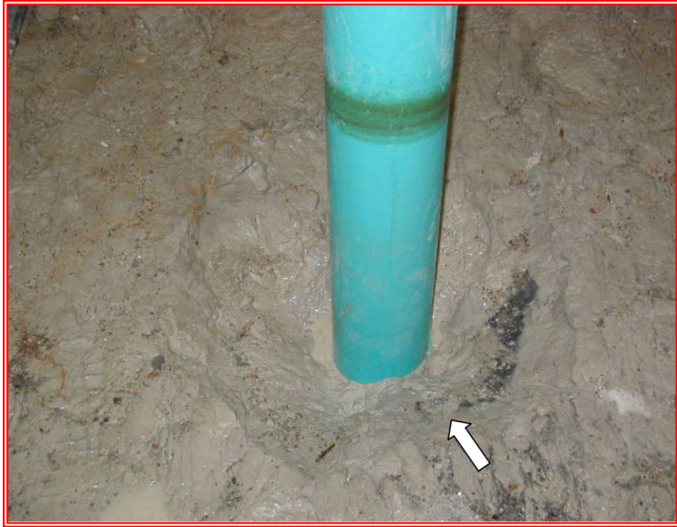
FIG 11 Scour Hole Geometry for Test 3
