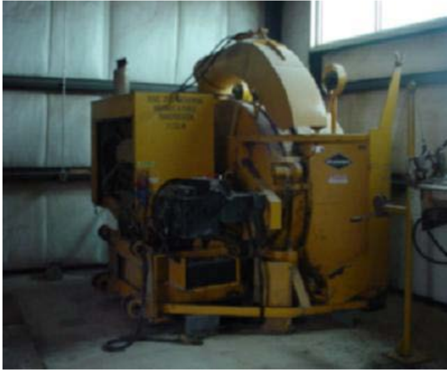
Figure 7-8. Snow Blower Is an Attachment that Is Used to Remove Large Quantities of Snow.
